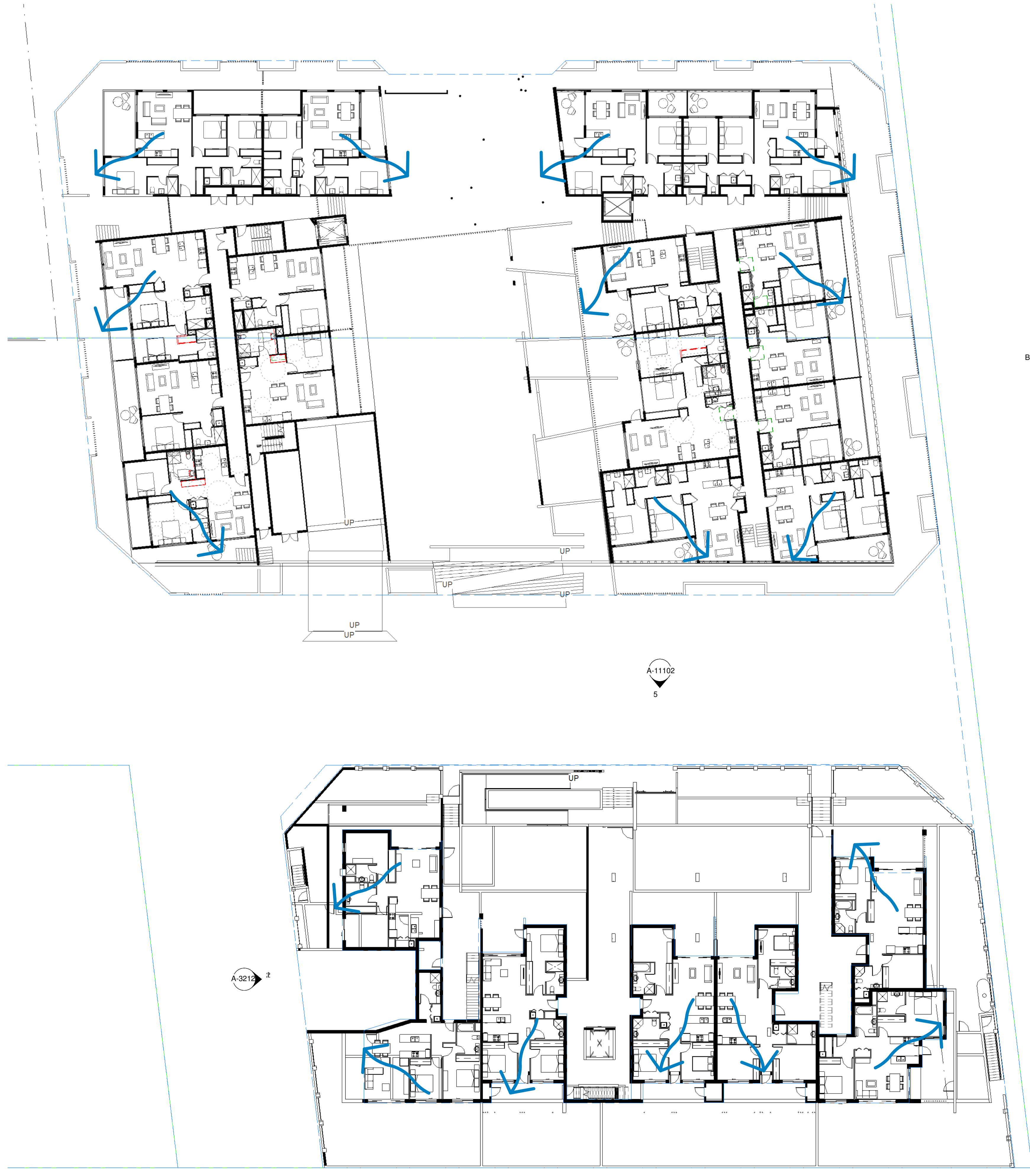
1 GROUND FLOOR - CROSS VENTILATION 1:200
